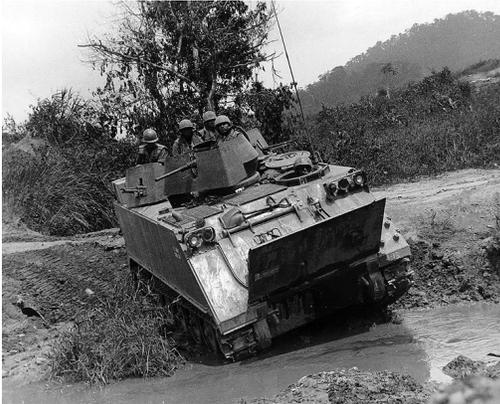
US Army variant had a .50 cal plus twin M-60s with armor around them. Our tracks had .50 cal. turret but the M-60 was on a quick release mount. Sometimes we also had an XM-148 drum-fed grenade launcher.
