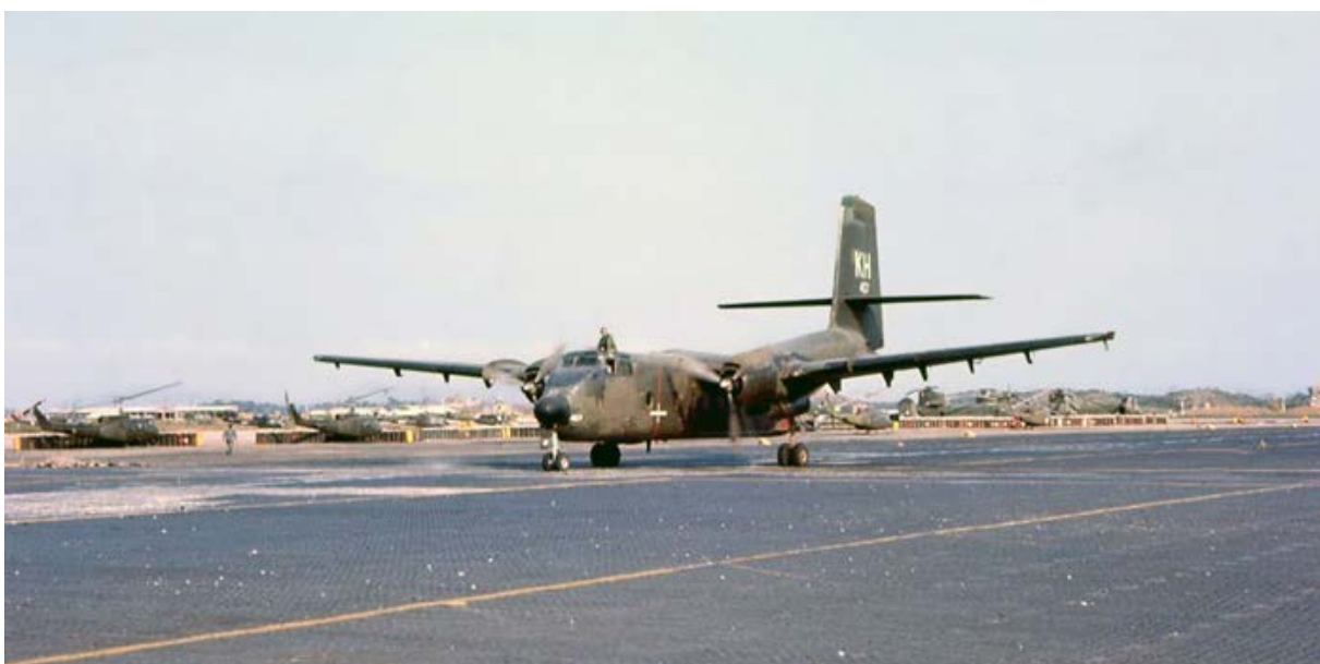
Binh Thuy Air Base flight line. Australian Caribou STOL taxis along PSP apron. MSgt Summerfield: 10
