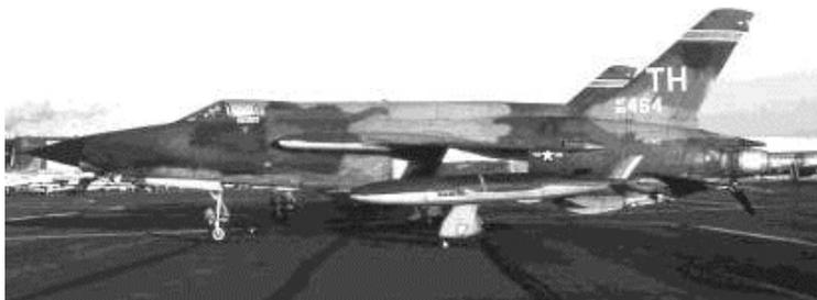
*The dorsal hump that distinguished the T-Stick II conversions is clearly evident in this post-war photograph of an F-105D. Source: U.S. Air Force*
