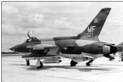
*This F-105D is a Thunderstick II conversion, which is easily distinguished from the standard -D model by the backbone electronics bay fairing from the cockpit to the vertical stabilizer. Thunderstick II allowed the aircraft to deliver ordnance under most flight conditions (speed, altitude and attitude) by automating weapons delivery and piloting. Source: U.S. Air Force*
