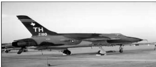
*The avionics hump on the F-105D actually improved the aircraft's lateral stability. Source: U.S. Air Force.*
