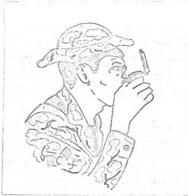
FIGURE 21 . COMPASS POSITION FOR SIGHTING
