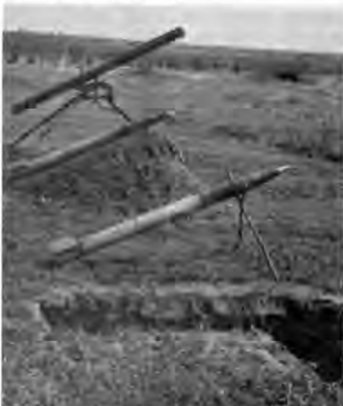
Display of the three basic methods used by the Viet Cone to launch rockets: launch tube, earth embankment, and crossed sticks
