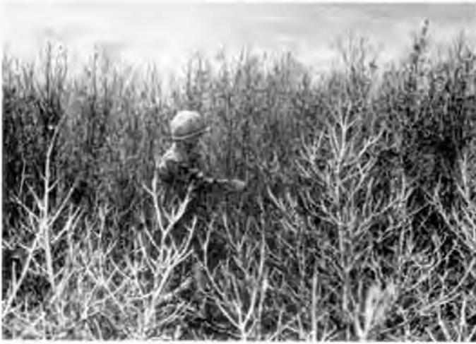
A Vietnamese soldier sprays fuel oil on dense foliage to determine the effectiveness of defoliation by fire. This failed because the fire would not keep burning
