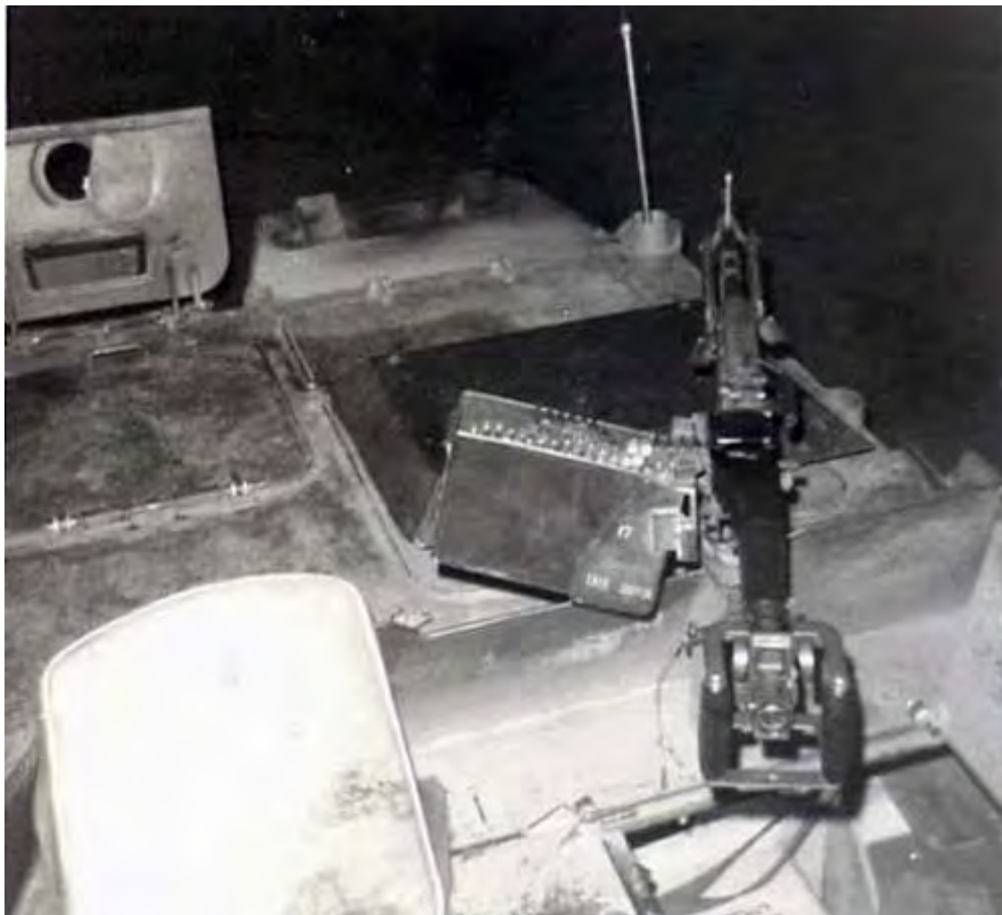
38. Phan Rang AB, V100, M60 with aircraft trigger system.
