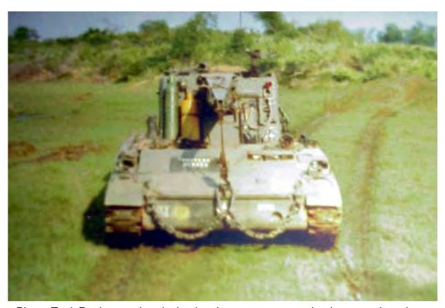
Photo: Tank Retriever arrives by land and prepares to enter the river to retrieve the APC.
