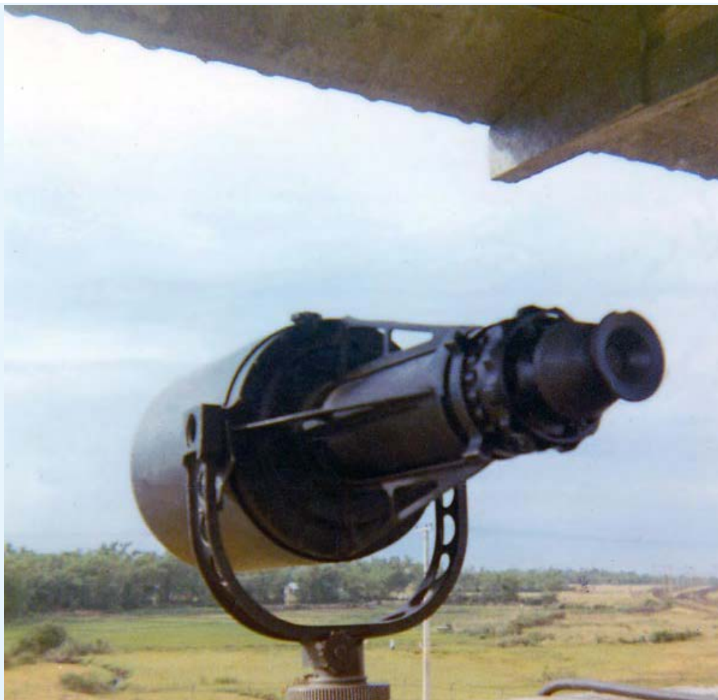
4a. Đà Nẵng AB, Perimeter Tower, Alpha-3, Starlite scope (TVS-4 or TVS-4A "Night Observation Device" Starlite 'scope). Photo by Konrad Kottke. 1971-1972.
