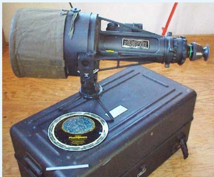
4b. Starlite scope: TVS-4 or TVS-4A "Night Observation Device" Starlite 'scope.
