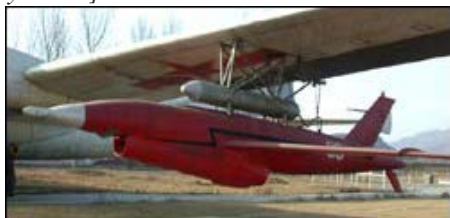
The Chang Hong-1 UAV, a reverse-engineered and heavily-modified replica of a captured USAF AQM-34N Firebee drone.
