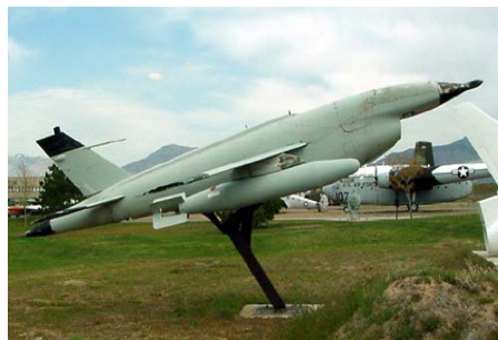
Photo left: China developed the CH-1 by reverse-engineering US Firebee reconnaissance AQM-34 drones recovered during the Vietnam War.
