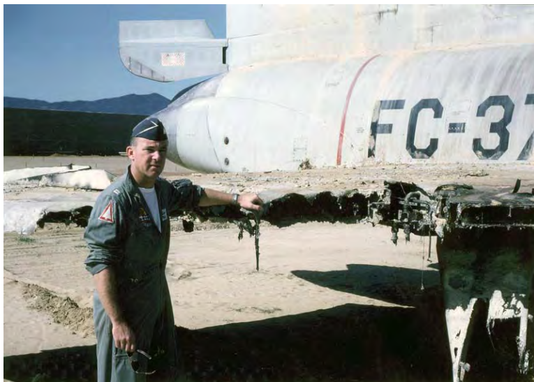
Photo-3, left, by: Capt Roger Pile, standing by an F102 which had the leading edge of the wing melted from the heat of a C130 burning.
