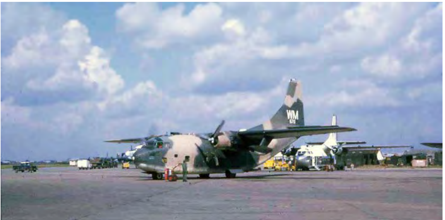
Binh Thuy Air Base flight line. C-123 prepares to start second engine, as crewman standsby with extinguisher. MSgt Summerfield: 12
