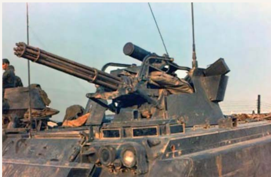
9. Bien Hoa AB, US Army M163 VADS 20-mm Gatling Gun (Vulcan), part of the Vulcan Combat Team. Photo by Ernest Govea.
