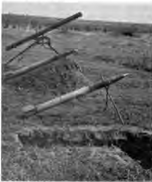
Display of the three basic methods used by the Viet Cong to launch rockets: launch tube, earth embankment, and crossed sticks
