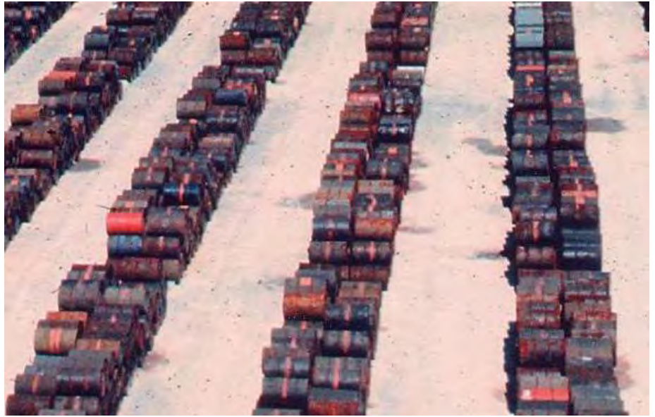
Note the photo left, where the sand is discolored by leaking barrels.
