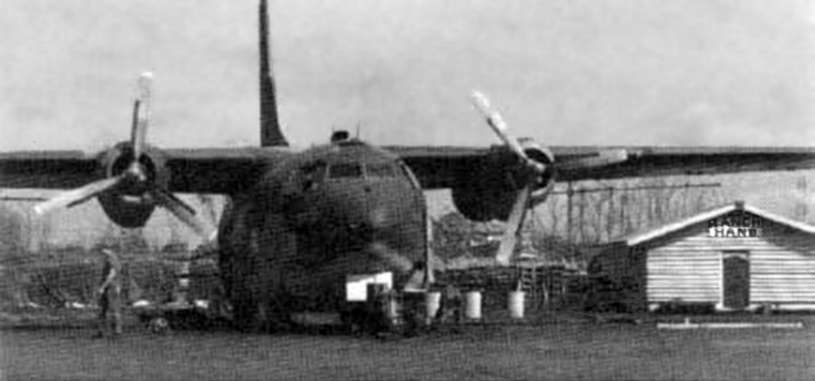
A Ranch Hand UC-123 with spraying arms under the wings at Tan Son Nhut
