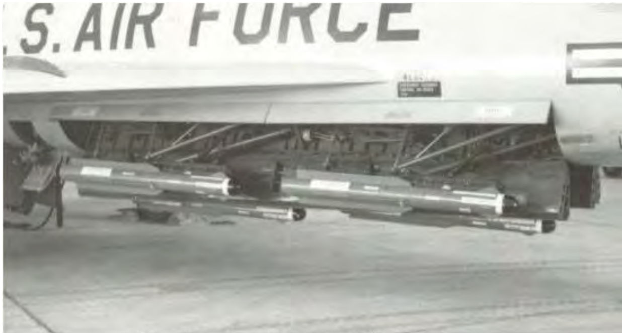
Internal weapons bays on the F-102 Delta Dagger
