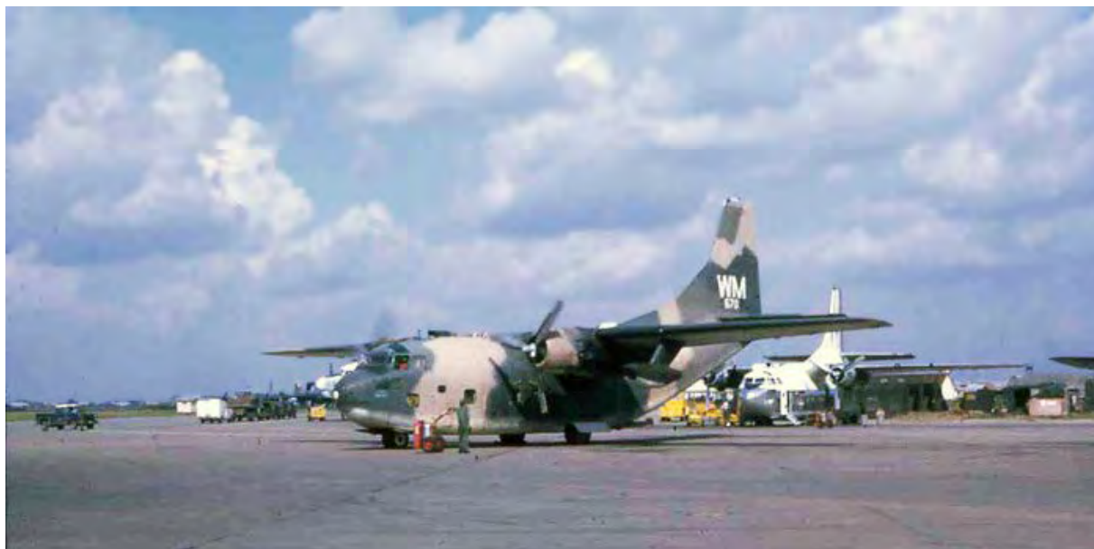
Binh Thuy Air Base flight line. C-123 prepares to start second engine, as crewman standby with extinguisher. MSgt Summerfield: 12
